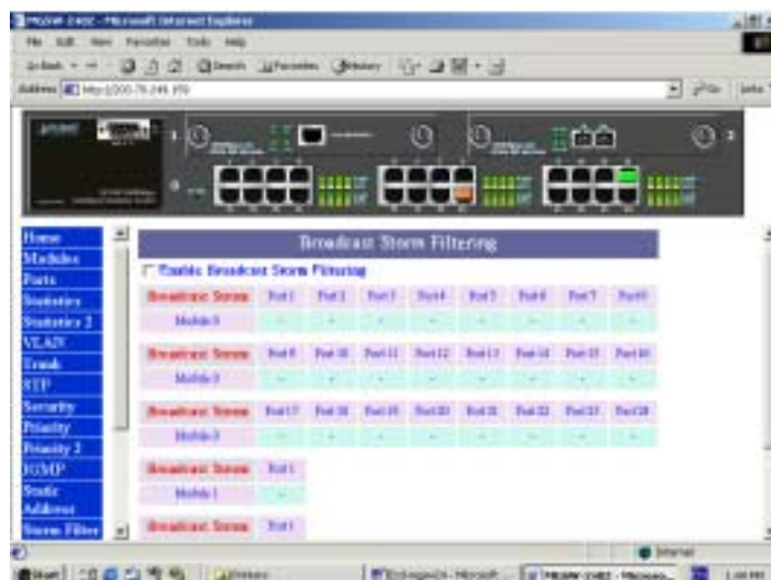
Figure 3-14 The Broadcast Storm Filter page
